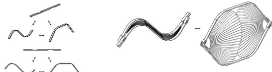
FIG 1A. Concept of snapping-induced motion with Weakening-induced bands (double induced)
